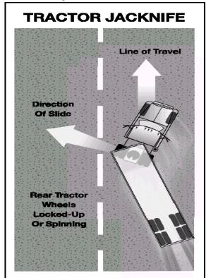
the trailer push the towing vehicle sideways, causing a sudden jackknife. See Figure 2.19.
