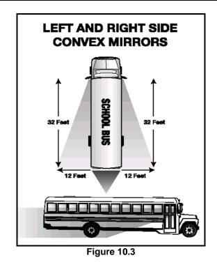
right side of the bus, including the service door and front wheel area. The mirror presents a view of people and objects that does not accurately reflect their size and distance from the bus. The driver must ensure that these mirrors are properly adjusted.
